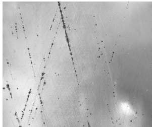
Figure 2. Discontinuities on the side surface of the can after the sulfate test
